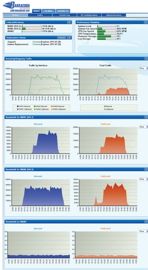
The Barracuda Link Balancer routes and manages traffic across multiple Internet connections from one or multiple service providers.
